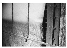
Competitive roll with low tensile strength causes the media to "neck" and pull out of the side channels. Unfiltered air is allowed to bypass the media.
