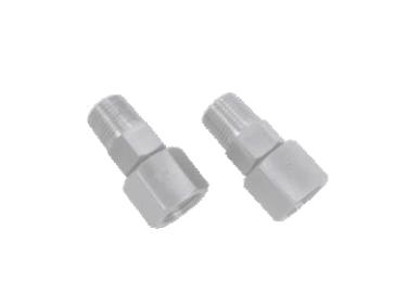
Universal Adaptor (Swivel Adaptor) facilitates the positioning of the Instrument during installation. Generally offered in material like SS304, SS316, Monel etc. (Other material on request). Standard connection is 1/2" NPT(F) x 1/2" NPT(M) (other connection on request)
