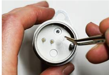
2. Inspect, and clean surface
