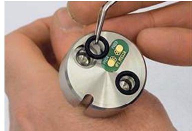
5. Place new o-rings, assemble the product
