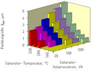
Adjustable Particle Sizes in Dependency on Saturator Flowrate and Saturator Temperature (DEHS)
