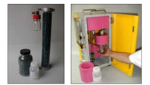
Left: Dismounted Nuclei Source (Atomizer and Diffusion Dryer) for Replacing Dessicant (Silicagel) through the Inlet on the Top Right: Removing Saturator Vessel for Refilling with Particle Material
