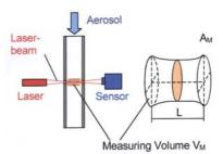
Under the assumption of monodisperse particle size distribution this optical reading technique delivers by means of the Lambert-Beer law both particle size and concentration. Via standard serial interface at the PAM 510/S and special software PAMWin measuring data can be transferred to a PC for further evaluation and presentation.
