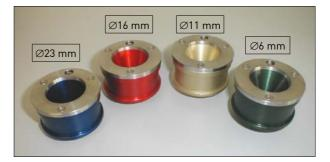
Colour-coded adapters for clamping the sample
